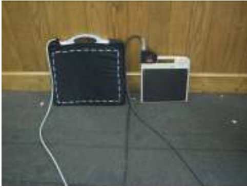
Fig. 2. 14"x 17" and 9" x 11" sensor panels for obtaining digital radiographs.
