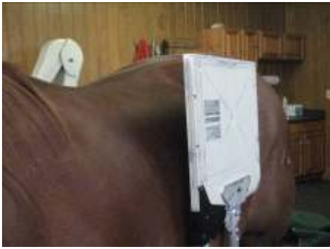
Fig. 3. Close placement of the sensor panel to the trunk of the horse.
