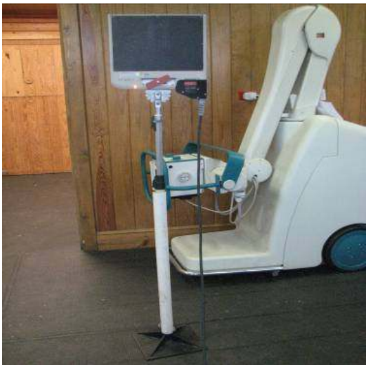
Fig. 1. Movable stand for direct digital capture sensor panel and high output radiographic generator e .
